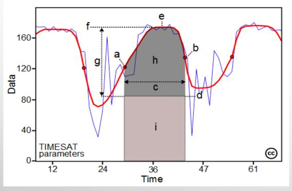
FIGURE 1. SOME OF THE SEASONALITY PARAMETERS GENERATED IN TIMESAT: (A) BEGINNING OF SEASON, (B) END OF SEASON, (C) LENGTH OF SEASON, (D) BASE VALUE, (E) TIME OF MIDDLE OF SEASON, (F) MAXIMUM VALUE, (G) AMPLITUDE, (H) SMALL INTEGRATED VALUE, (H+I) LARGE INTEGRATED VALUE. THIS FIGURE IS LICENSED UNDER A CREATIVE COMMONS ATTRIBUTION-NONCOMMERCIAL-NODERIVS 2.5 SWEDEN LICENSE. IT IS FREE TO COPY AND USE IN OTHER WORK
